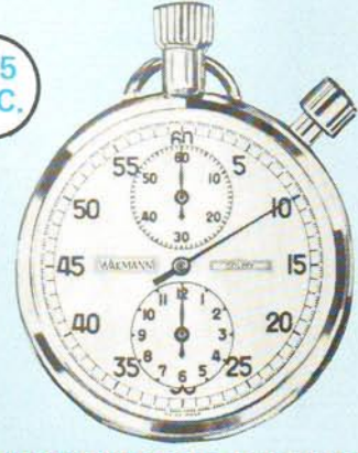
1/5 SECOND TIME OUT TIMER WITH 12 HOUR TOTALIZER Lower totalizer registers up to 12 hours; the upper one registers up to 60 minutes. Start, stop and re-start by depressions of crown. All hands fly back by depressing side button. 938 . . . 7 Jewels 338 . . . (Same with 1 Jewel)
